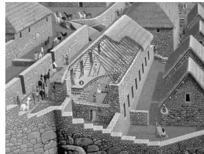
Figure 10. Experts are still debating the types of Inca roof structures of Machu Picchu. This National Geographic magazine portrayal represents the most likely structure to have been able to support the heavy thatched roofs.
